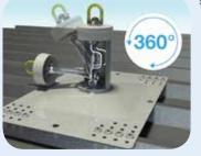
**360° protection :** In the event of a fall, the Söll Fusion® Roof Anchor Post collapses in the direction of the force, the built-in, energy-absorbing component activates and the base remains securely attached to the roof surface.
